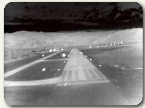
EVS-600 Shows Runway lighting
